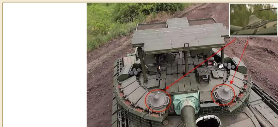
Image 1 - Russian communications jammer mounted on T-90.
