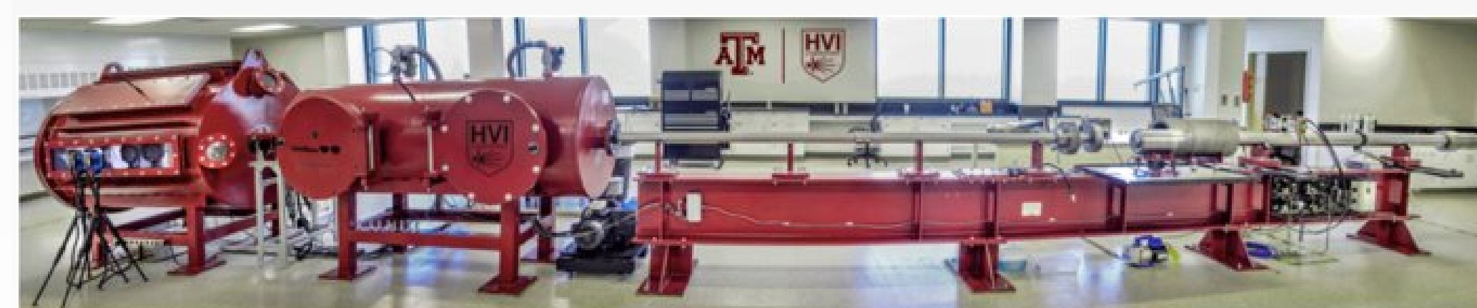
Two-stage light gas gun at Texas A&M
