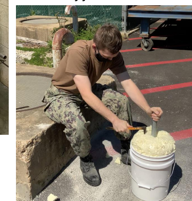
MIDN Budan performing a rigid foam dig test, where a midshipman is timed to see how long it takes to unscrew a rod from a bucket covered a certain amount of foam.
