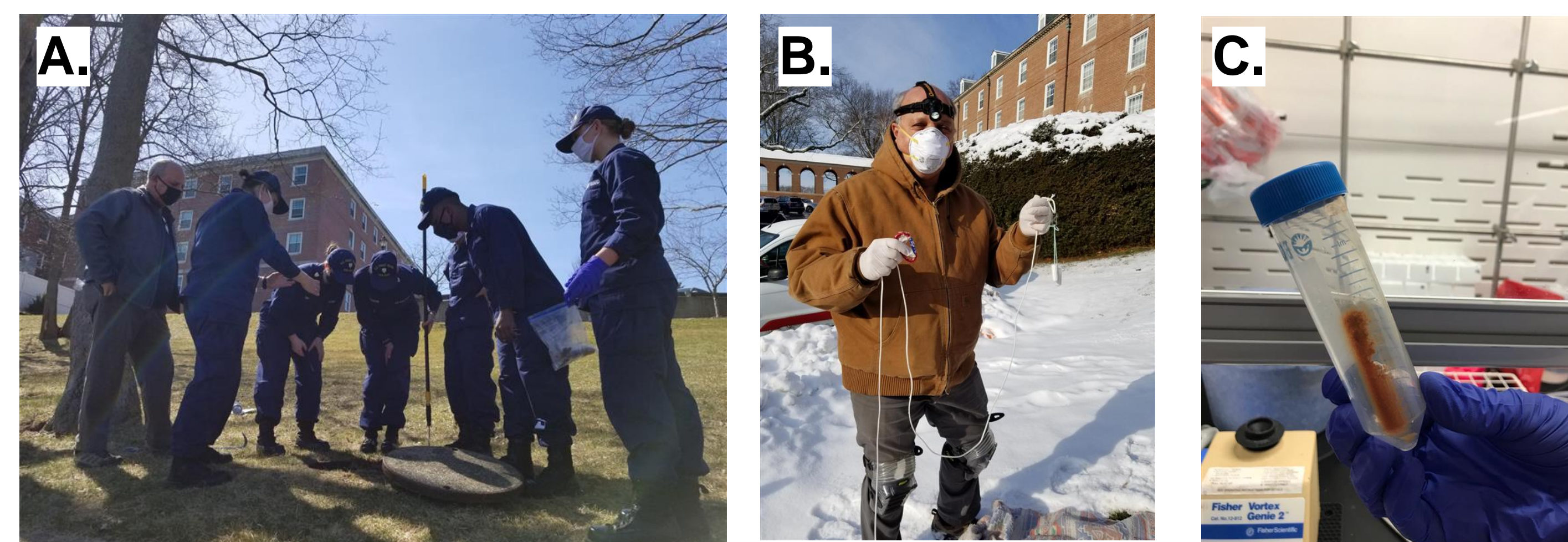
Figure 1. Method of sewage sample retrieval and extraction. A. Samples are placed in raw sewage manholes. B. Absorbent material is placed into the manhole. C. During extraction, virus particles are absorbed onto magnetic Nanotrap beads and a neodymium magnet is used to purify virus from the remainder of the sewage sample. D. Following this step, RNA is extracted by the Qiagen Viral kit as per manufacturer's instructions.
