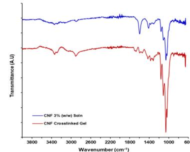
**Figure 3.** Fourier transform infrared (FTIR) spectra of 3% cellulose nanofiber (CNF) solution (blue) and EDC crosslinked CNF fiber (red).
