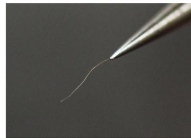
**Figure 2.** Photo of air-dried cellulose nanofiber hydrogel fiber.
