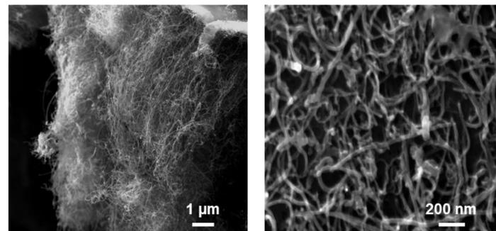
**Figure 5.** 3-D integrated CNT-biopolymer high surface area nano-architecture. Inter-penetrating CNT network upholds toughness, tensile strength, conductivity.
