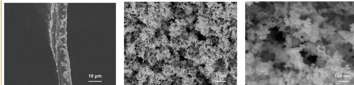
**Figure 9.** Scanning electron microscope images of cellulose nanofiber biotemplated fibers crosslinked with 1-ethyl-3-(3-dimethylaminopropyl) carbodiimide hydrochloride (EDC) with a diamine linker. Air dried fibers were equilibrated in 0.5 M  $K_2PtCl_6$  and reduced with 1 M  $NaBH_4$ .
