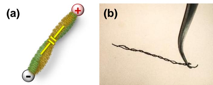
**Figure 4.** (a) Intertwined CNT-biopolymer multi-functional fibers serving as both textile fiber and capacitive energy storage material. (b) Intertwined CNT-alginate fibers precipitated from 10%, 1:1 (w/w) CNT:alginate solution extruded into 10 M  $CaCl_2$ .
