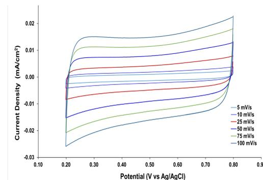
**Figure 6.** Cyclic voltammetry in 0.5 M KCl of CNT-PVA fiber serving as textile fiber and capacitive storage material. Specific capacitance of 11.4 mF/cm<sup>2</sup>.
