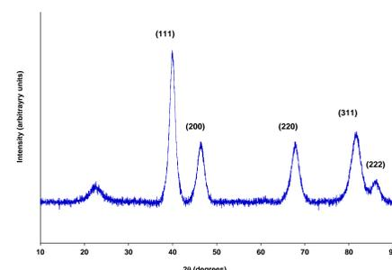
**Figure 8.** X-ray diffraction (XRD) spectra. Platinum peaks were indexed to Joint Committee on Powder Diffraction Standards (JCPDS) reference number 01-087-0640 for platinum.
